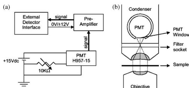
Fig. 2. (a) Schematic representation of the connection between the PMT power supply, the variable resistor, PMT, Pre-Amplifier and the external detector interface, on with the final signal was attached for producing a scanning image. (b) Scheme of the light path and the mounting positions of the devices.
