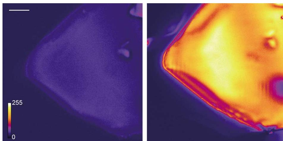
Fig. 4. Crystals of  $\text{KH}_2\text{PO}_4$  mounted in immersion oil. Images collected by forward and backward detection. Band pass filter D455/30, for both back and forward directions, using 910 nm excitation. Scale bar 25  $\mu\text{m}$ .
