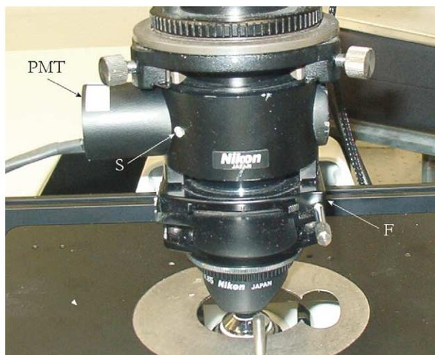
Fig. 3. Photograph of our detector installed behind the condenser of the TE300. PMT—the Hamamatsu H957 photomultiplier module; S—locking screw to secure it in place; F, filter holder (originally holder for polarizer). The objectives are visible beneath the stage.
