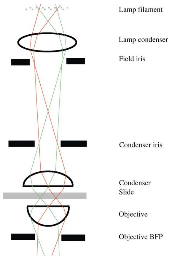
Fig. 1. Ray paths in an inverted microscope set up for Köhler illumination. Two separate positions of the scanning beam are shown (red and green). At the plane of the condenser iris (condenser BFP) the position of the beam is the same whichever spot is being scanned. At the plane of the field iris the scan pattern is imaged, and then at the lamp filament we have a BFP, and the beam position is again independent of the scan.
