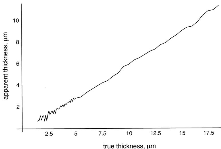
Fig. 5. The calculated dependence between real and apparent thickness, for  $\lambda = 488$  nm and 0.85 NA.
