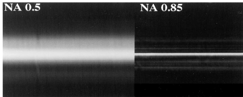
Fig. 7. Experimental  $xz$  images produced using lenses of numerical aperture: (a) 0.5, and (b) 0.85,  $\lambda = 488$  nm.
