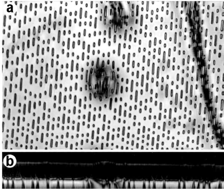
Fig. 2. (a) Surface view (extended focus image) of the upper surface of a faulty compact disk. Several blishes are visible in the varnish coating. (b)  $xz$  section taken from the midline of the image in (a). The images of the pits are very complex, emphasizing the need to measure the coating thickness in smooth regions. The perturbing effect of the 'blister' in the coating is also evident in the apparent depression of the alumined surface beneath it.
