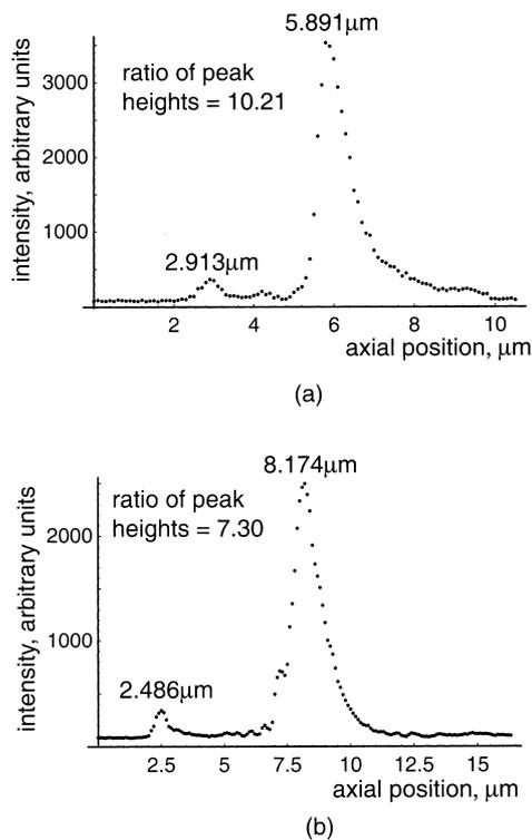
Fig. 3. Measured axial intensity variation for  $\lambda = 488$  nm and 0.85 NA on two disks with different coating thicknesses. The data points correspond to individual voxel values, the spacing of which is limited by the precision of the stepper motor. The positions of the peaks were therefore derived by parabolic interpolation from the data points. The ratio of the peak heights is another feature which can be compared with theoretical predictions.
