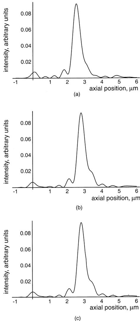
Fig. 4. Calculated axial image for  $\lambda = 488$  nm and 0.85 NA for coatings of thickness (a) 4.5  $\mu\text{m}$ , (b) 5.0  $\mu\text{m}$ , (c) 5.5  $\mu\text{m}$ . The position of the top reflection (left-hand peak) is seen to shift as a result of interference effects.
