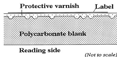
Fig. 1. Diagrammatic view of the structure of a compact disc.
