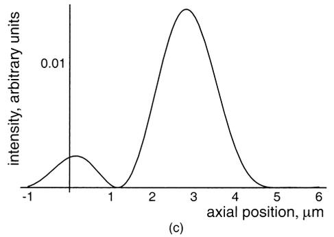
Fig. 6. Calculated axial image for  $\lambda = 488$  nm and 0.85 NA for coatings of thickness (a) 9.0 mm, (b) 9.5 mm, (c) 10.0 mm. In (b) a double peak is seen, while peak hopping is observed between (a) and (b).
